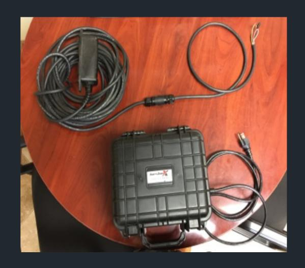
Locking, gender specific cable connections ensure correct attachment and also allow the system to operate in the absence of the intrinsically safe controller (by-pass mode).
