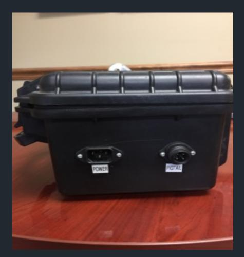
An intrinsically safe controller circuit enclosed in a waterproof polypropylene case, with waterproof connections for wiring to the pump, wiring to the remote hand controller and AC power in.
